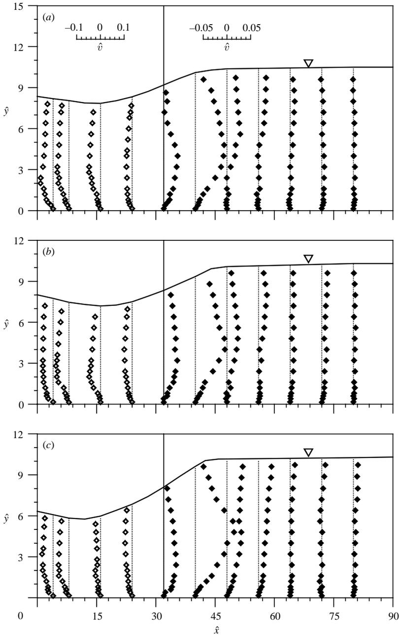
FIGURE 3. Vertical profiles of  $\hat{v}$  for  $U = 1.435 \text{ m s}^{-1}$ ,  $L = 0.4 \text{ m}$  and  $b = 12.5 \text{ mm}$ :
