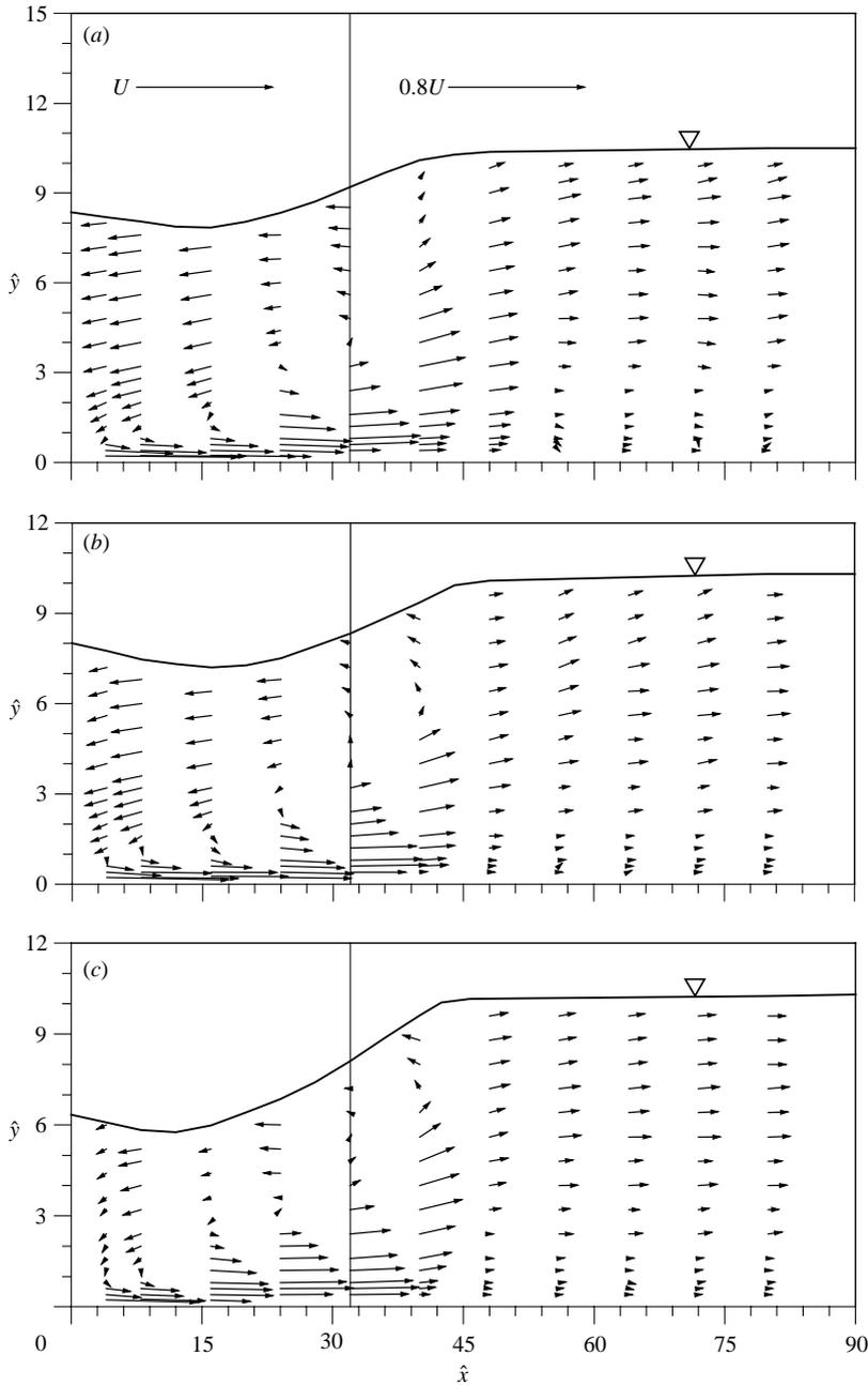
FIGURE 4. Non-dimensional velocity vectors for  $U = 1.435 \text{ m s}^{-1}$ ,  $L = 0.4 \text{ m}$  and  $b = 12.5 \text{ mm}$ :
