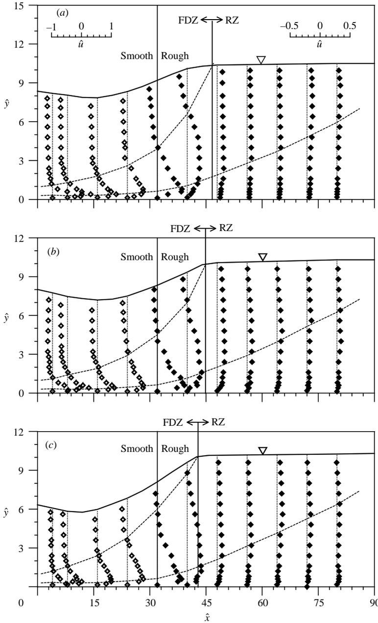
FIGURE 2. Vertical profiles of  $\hat{u}$  for  $U = 1.435 \text{ m s}^{-1}$ ,  $L = 0.4 \text{ m}$  and  $b = 12.5 \text{ mm}$ : (a)  $\epsilon = 0.8 \text{ mm}$ , (b)  $\epsilon = 1.86 \text{ mm}$  and (c)  $\epsilon = 3 \text{ mm}$  (FDZ and RZ refer to the fully developed and recovering zones, respectively).
