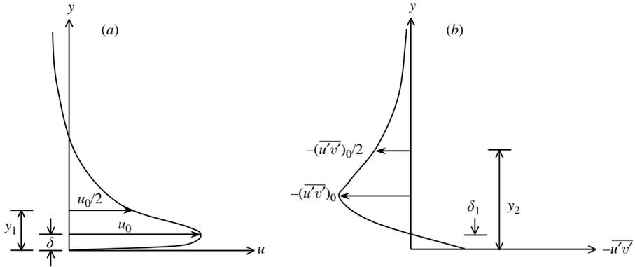
FIGURE 10. (a) Schematic velocity profile and (b) schematic Reynolds stress profile.
