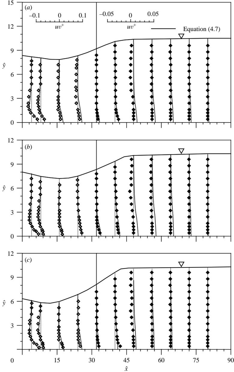
FIGURE 7. Vertical profiles of Reynolds stress  $uv^+$  for  $U = 1.435 \text{ m s}^{-1}$ ,  $L = 0.4 \text{ m}$  and  $b = 12.5 \text{ mm}$ : (a)  $\varepsilon = 0.8 \text{ mm}$ , (b)  $\varepsilon = 1.86 \text{ mm}$  and (c)  $\varepsilon = 3 \text{ mm}$ .
