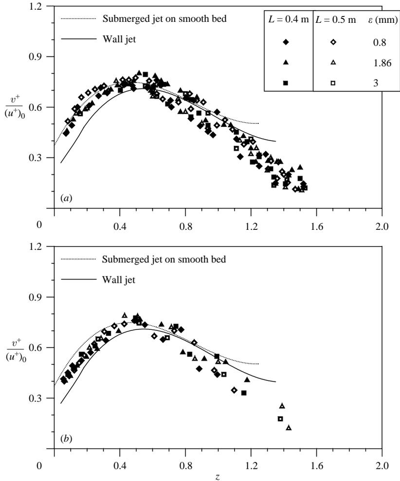
FIGURE 16. (a) Similarity of distributions of  $v^+$  in fully developed zone of smooth beds for different downstream  $\epsilon$  and  $L$  ( $L = 0.4$  m (data range:  $3.3 \leq \hat{x} \leq 20$ ) and  $0.5$  m (data range:  $3.3 \leq \hat{x} \leq 26.7$ )) and (b) similarity of distributions of  $v^+$  in fully developed zone of rough beds for different  $\epsilon$  and  $L$  ( $L = 0.4$  m (data range:  $26.7 \leq \hat{x} \leq 40$ ) and  $0.5$  m (data range:  $33.3 \leq \hat{x} \leq 40$ )).
