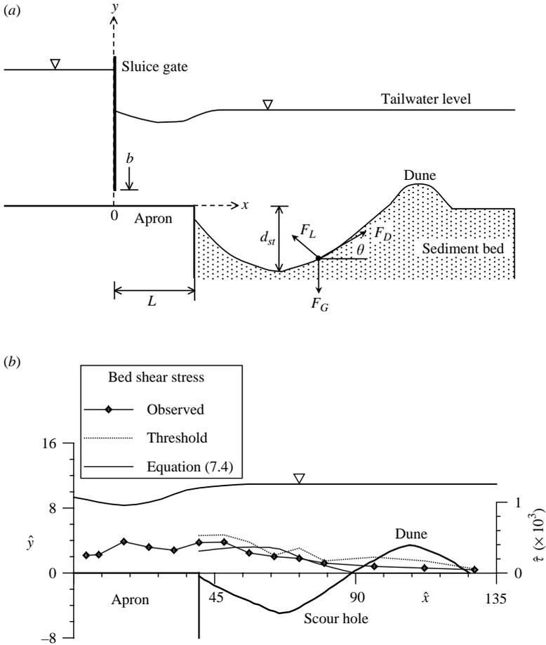
FIGURE 18. (a) Schematic diagram of scour downstream of an apron due to a submerged jet issuing from a sluice opening and (b) variations of bed shear stress  $\hat{\tau}$  on scoured beds for  $U = 1.435 \text{ m s}^{-1}$ ,  $L = 0.4 \text{ m}$ ,  $b = 12.5 \text{ mm}$  and  $d_{50} = 0.8 \text{ mm}$ .
