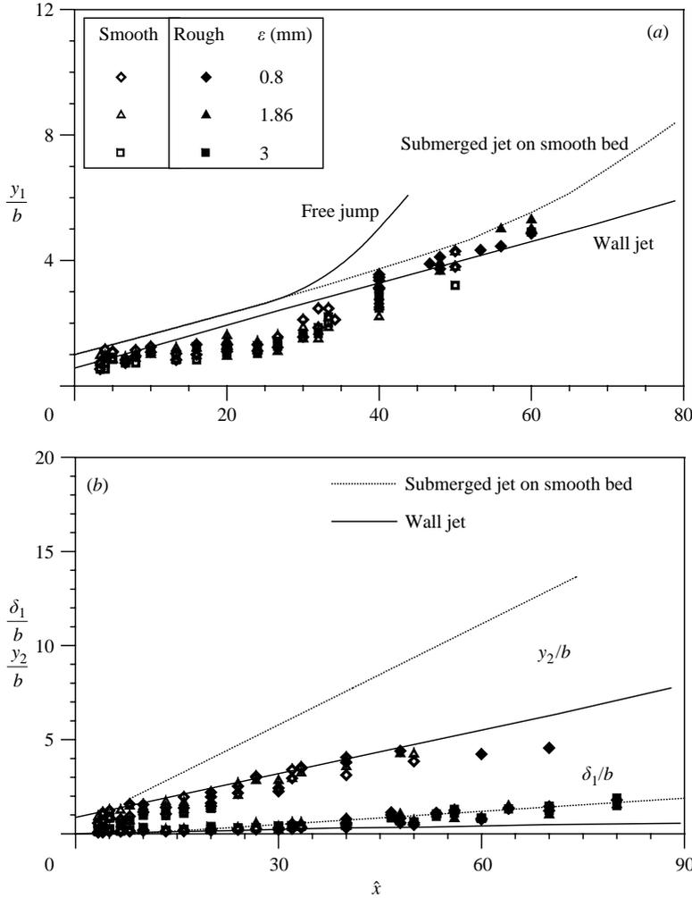
FIGURE 17. Variations of (a)  $y_1/b$  and (b)  $\delta_1/b$  and  $y_2/b$  with  $\hat{x}$  for different  $\epsilon$  and  $L = 0.5$  m.
