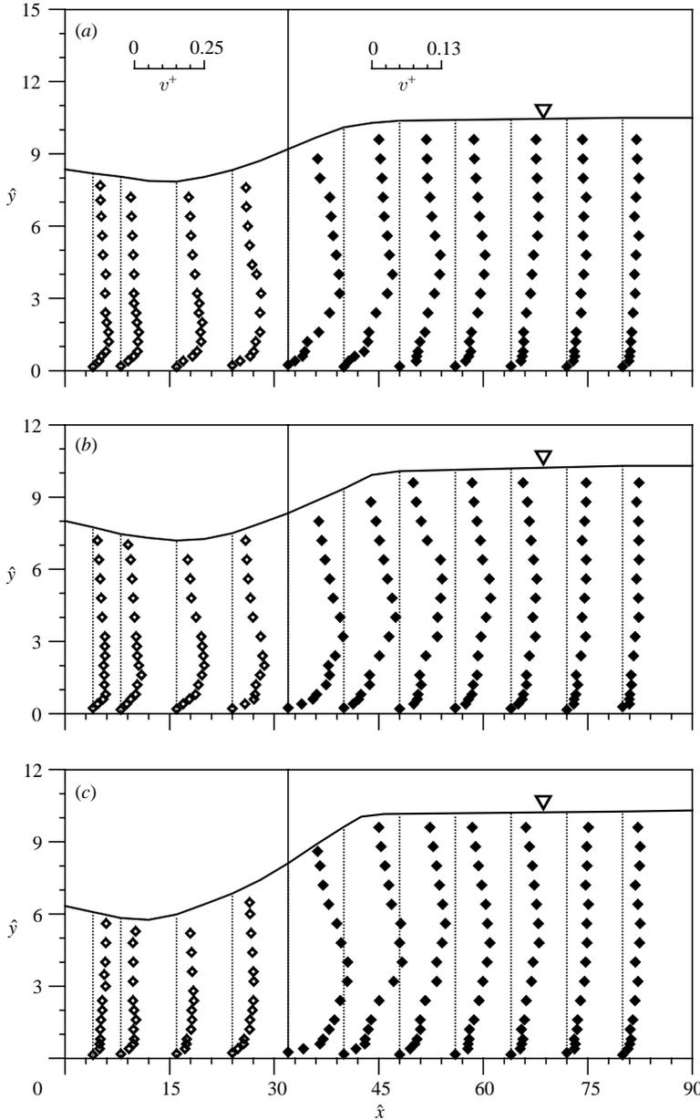
FIGURE 6. Vertical profiles of  $v^+$  for  $U = 1.435 \text{ m s}^{-1}$ ,  $L = 0.4 \text{ m}$  and  $b = 12.5 \text{ mm}$ : (a)  $\varepsilon = 0.8 \text{ mm}$ , (b)  $\varepsilon = 1.86 \text{ mm}$  and (c)  $\varepsilon = 3 \text{ mm}$ .
