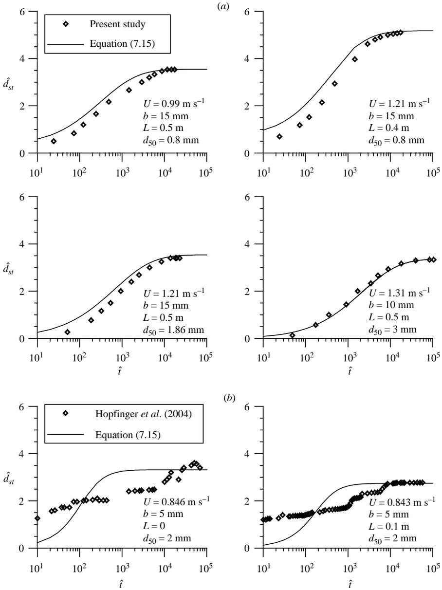
FIGURE 20. Comparisons of computed and experimental time-variation of scour depth ( $\hat{d}_{st}$  versus  $\hat{t}$ ): (a) data of present study and (b) data of Hopfinger *et al.* (2004).
