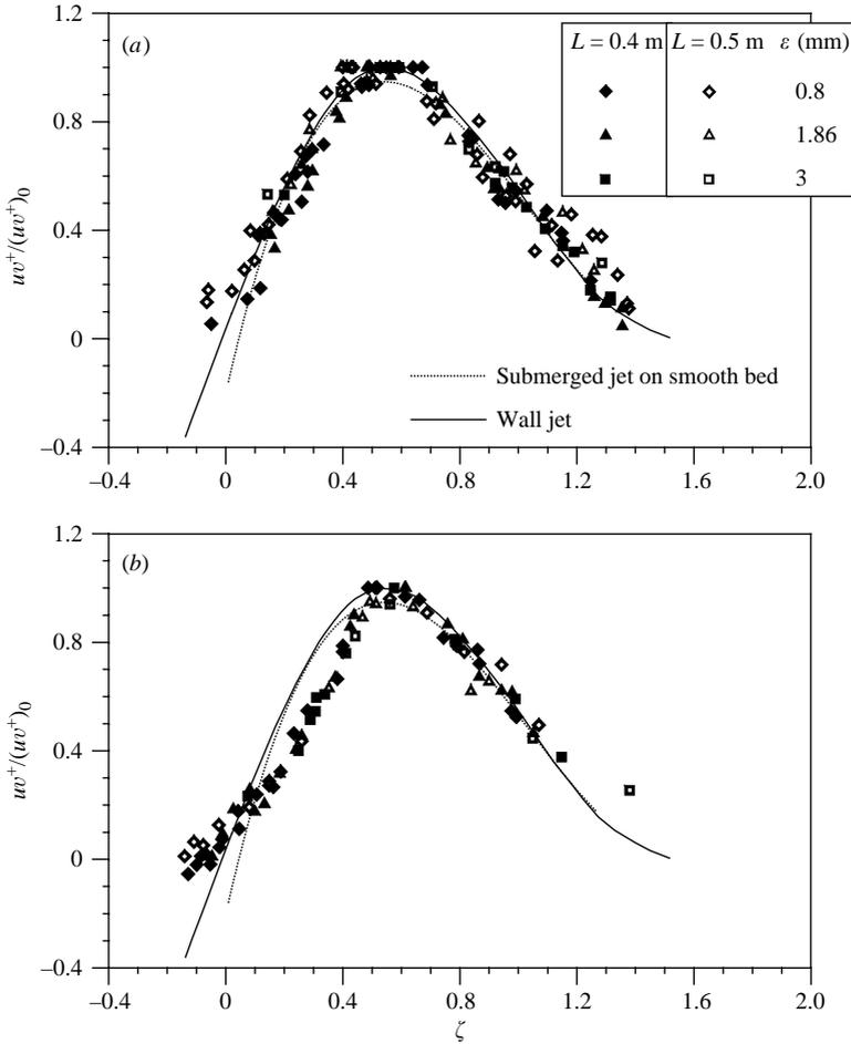
FIGURE 14. (a) Similarity of distributions of  $uv^+$  in fully developed zone of smooth beds for different downstream  $\epsilon$  and  $L$  ( $L=0.4$  m (data range:  $3.3 \leq \hat{x} \leq 20$ ) and  $0.5$  m (data range:  $3.3 \leq \hat{x} \leq 26.7$ )) and (b) similarity of distributions of  $uv^+$  in fully developed zone of rough beds for different  $\epsilon$  and  $L$  ( $L=0.4$  m (data range:  $26.7 \leq \hat{x} \leq 40$ ) and  $0.5$  m (data range:  $33.3 \leq \hat{x} \leq 40$ )).
