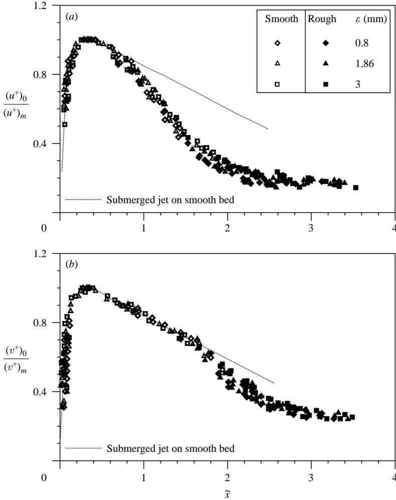
FIGURE 12. (a) Dependence of  $(u^+)_0/(u^+)_m$  and (b) dependence of  $(v^+)_0/(v^+)_m$  on  $\tilde{x}$  for different  $\epsilon$  and  $L = 0.5$  m.
