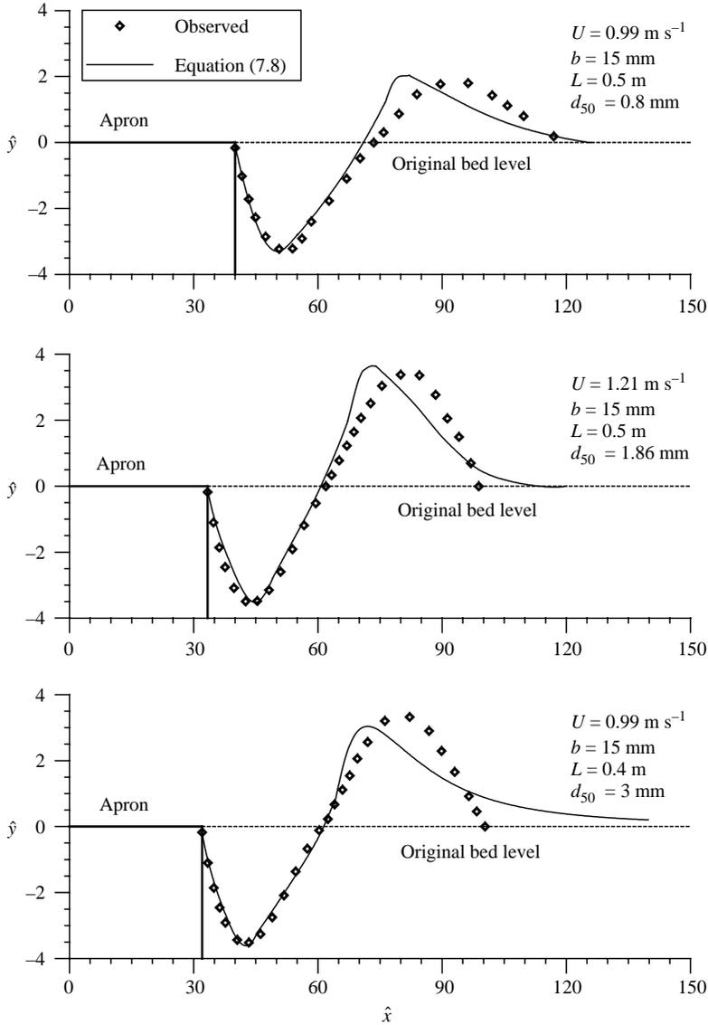
FIGURE 19. Comparisons of computed and experimental scour profiles.
