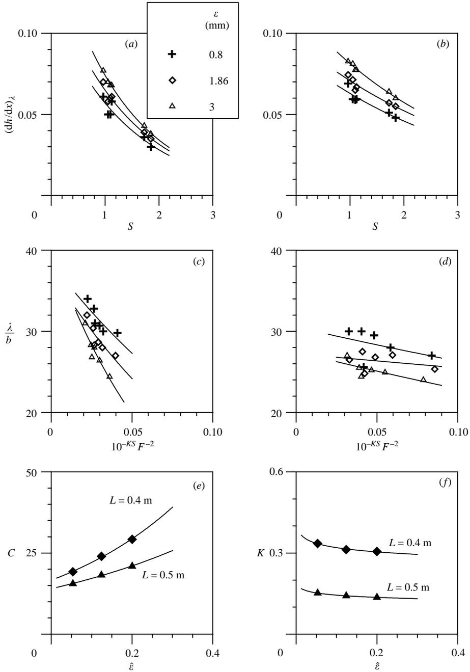
FIGURE 9. (a)  $(dh/dx)_\lambda$  as a function of  $S$  for  $L=0.4$  m, (b)  $(dh/dx)_\lambda$  as a function of  $S$  for  $L=0.5$  m, (c)  $\lambda/b$  as a function of  $10^{-KS} F^{-2}$  for  $L=0.4$  m, (d)  $\lambda/b$  as a function of  $10^{-KS} F^{-2}$  for  $L=0.5$  m, (e) variation of  $C$  with  $\hat{\epsilon}$  and (f) variation of  $K$  with  $\hat{\epsilon}$ .
