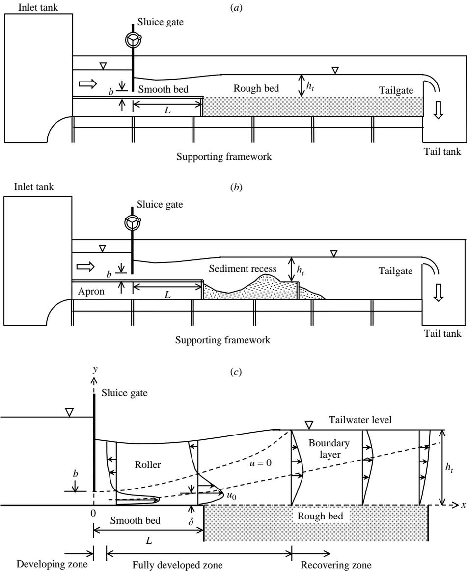
FIGURE 1. (a) Schematic diagram of the fixed bed experimental setup for a submerged wall jet on a rigid bed with abrupt changes of bed roughness, (b) schematic diagram of mobile bed experimental setup for scour downstream of an apron due to a submerged jet issuing from a sluice opening and (c) diagram showing the flow zones in a submerged wall jet.
