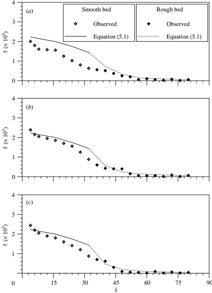
FIGURE 8. Horizontal distributions of bed shear stress  $\hat{\tau}$  for  $U = 1.435 \text{ m s}^{-1}$ ,  $L = 0.4 \text{ m}$  and  $b = 12.5 \text{ mm}$ : (a)  $\varepsilon = 0.8 \text{ mm}$ , (b)  $\varepsilon = 1.86 \text{ mm}$  and (c)  $\varepsilon = 3 \text{ mm}$ .
