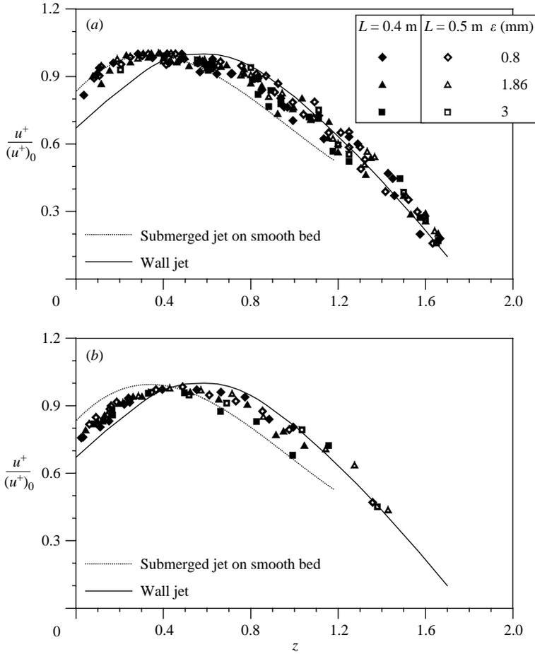
FIGURE 15. (a) Similarity of distributions of  $u^+$  in fully developed zone of smooth beds for different downstream  $\epsilon$  and  $L$  ( $L=0.4$  m (data range:  $3.3 \leq \hat{x} \leq 20$ ) and  $0.5$  m (data range:  $3.3 \leq \hat{x} \leq 26.7$ )) and (b) similarity of distributions of  $u^+$  in fully developed zone of rough beds for different  $\epsilon$  and  $L$  ( $L=0.4$  m (data range:  $26.7 \leq \hat{x} \leq 40$ ) and  $0.5$  m (data range:  $33.3 \leq \hat{x} \leq 40$ )).
