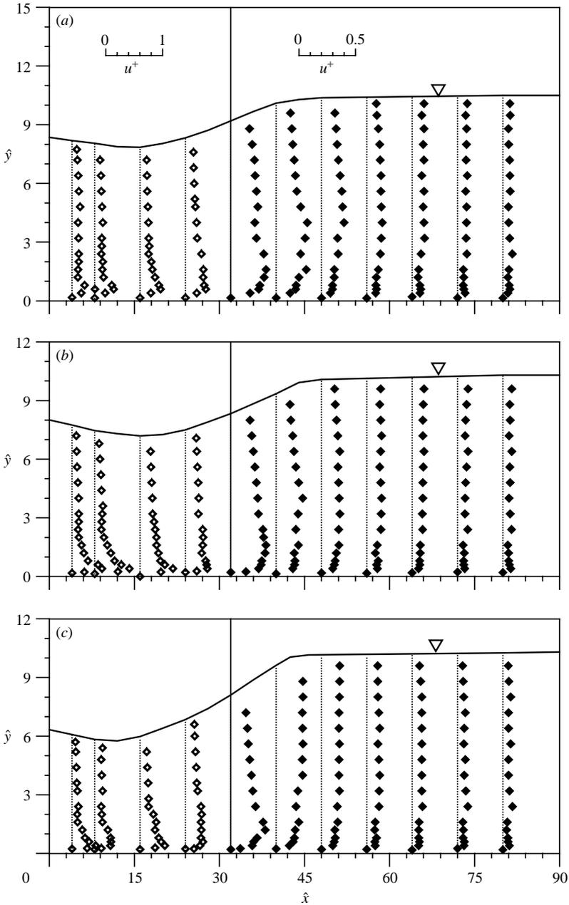
FIGURE 5. Vertical profiles of  $u^+$  for  $U = 1.435 \text{ m s}^{-1}$ ,  $L = 0.4 \text{ m}$  and  $b = 12.5 \text{ mm}$ : (a)  $\varepsilon = 0.8 \text{ mm}$ , (b)  $\varepsilon = 1.86 \text{ mm}$  and (c)  $\varepsilon = 3 \text{ mm}$ .
